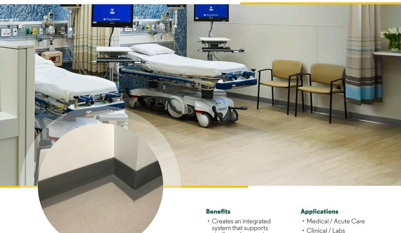
ECOsurfaces' Sanitary Base System creates an integrated floor system that supports sterile environments. By covering the joint at which two surfaces meet, moisture and germs are prevented from penetrating the area. The base is available in 7 colors. The system includes sanitary base, composition rubber underlayment, and Floor/Wall Contact Tape. Vertical seams must be cold welded (Bostik DUO-SIL is recommended).
