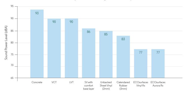
Testing was performed by Intertek, an independent IAS-certified lab in York, PA. The "SV with comfort base layer" sound level was provided from the manufacturer's published test data.
